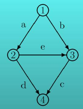
O/D w=(1,4) travel demand is  $d_w$ =6. Paths  $p_1$ =(a,c)  $p_2$ =(b,d). The user-optimized solution in path flows:  $x_{p1}^* = x_{p2}^* = 3$  The induced link flow pattern: The link travel costs:  $c_a$ =30  $c_b$ =53  $c_c$ =53  $c_d$ =30, and the user path travel costs:  $C_{p1}$ = $c_a$ + $c_c$ =83  $C_{p2}$ = $c_b$ + $c_d$ =83.
