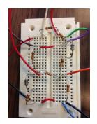
The voltages at nodes  $V_1$ ,  $V_2$ , and  $V_3$ , and the voltage across  $R_{sense}$  are measured using the 4 analog input channels of a National Instruments USB-6009 Multifunction I/O Data Acquisition system. The USB-6009 system was programmed using Labview running on a PC. From these measurements and the knowledge of the resistor values  $R_a$ ,  $R_b$ , and  $R_e$ , the link and path flows are calculated.
