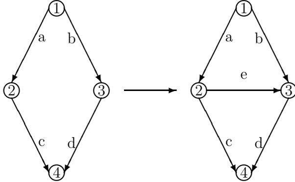
Figure 3: The Time-Dependent Braess Network Example with Relevance to the Internet
