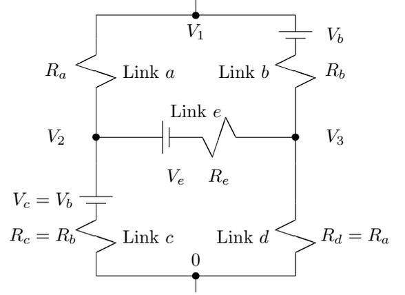
Fig. 2: Electrical Circuit Analogue for the Classical Braess Paradox
